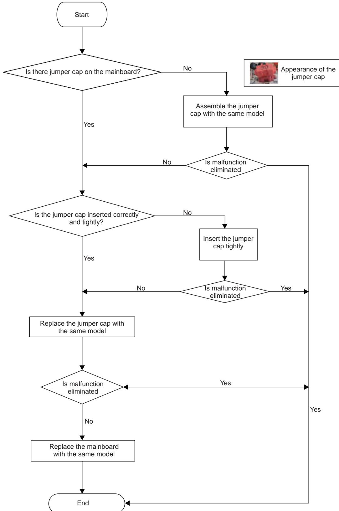
**5. Malfunction of Zero-crossing Inspection Circuit Malfunction of the IDU Fan Motor U8**
