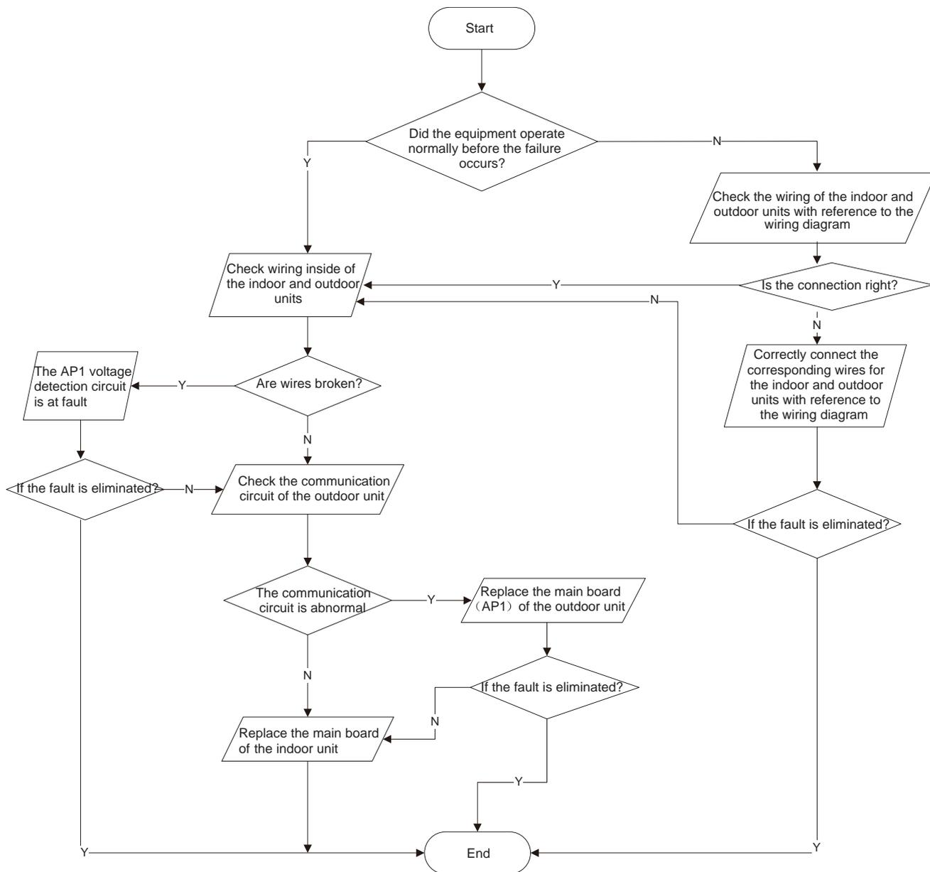
(9) Communication malfunction:(following AP1 for outdoor unit control board)
