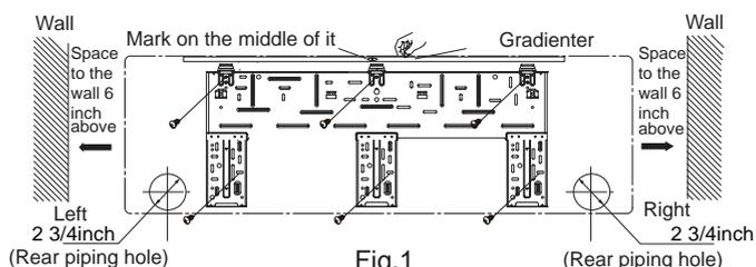
(2) Open a piping hole with the diameter of  $\Phi 2 \frac{3}{4}$  inch on the selected outlet pipe position. In order to drain smoothly, slant the piping hole on the wall slightly downward to the outdoor side with the gradient of  $5-10^\circ$ . (As show in Fig.2)
