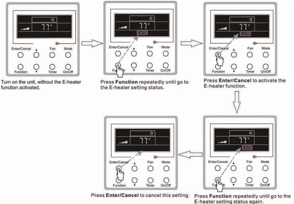
Fig.3.9.1 E-heater Setting
