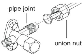
3. Tighten the union nut with torque wrench by referring to the sheet below.
