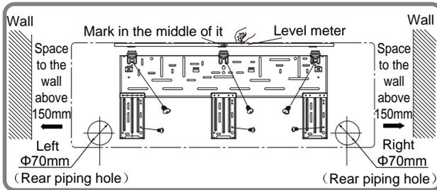
2. Open a piping hole with the diameter of  $\Phi 70$  on the selected outlet pipe position. In order to drain smoothly, slant the piping hole on the wall slightly downward to the outdoor side with the gradient of 5-10°.
