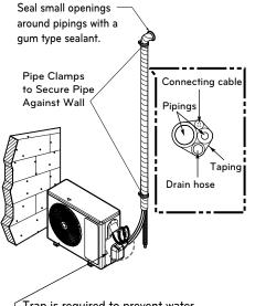
Trap is required to prevent water from entering into electrical parts.
