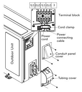
Figure 94: 180HEV Outdoor Unit - Electrical Connections
