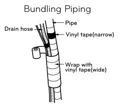
Figure 43: IDU Below ODU - Piping and Trap
