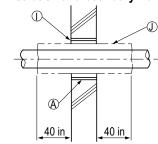
(A) Sleeve (B) Insulation CLagging DCaulk (E) Band (F) Water-resistant layer G Sleeve with edge HLagging (I) Mortar or other fire-resistant caulk (J) Fire-resistant insulation
