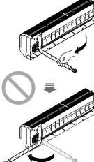
Do not bend tubing directly backwards or to the sides without bending downward first! This may cause damage!
