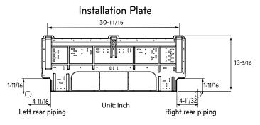
Figure 12: Drilling Piping Hole
