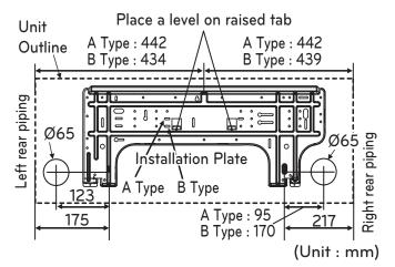
Figure 7: Installation Plate Screws
