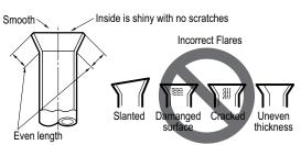
Piping Preparation / Piping Materials and Handling
