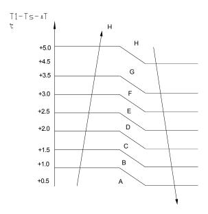
While the zones of A,B,C... are corresponding to different compressor running frequency.  $\Delta T$ =0  $^{\circ}$ C as default.
