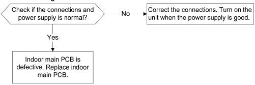
10.4.4 Fan speed has been out of control diagnosis and solution(E3)
