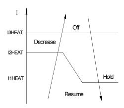
I3HEAT, I2HEAT,I1HEAT mean different running current value.
