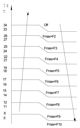
Fmax: The maximum operation frequency of compressor.
