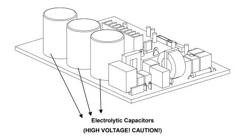
For other models, please connect discharge resistance (approx.100 $\Omega$  40W) or soldering iron (plug) between +, - terminals of the electrolytic capacitor on the contrary side of the outdoor PCB.
