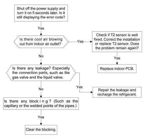
10.4.7 IPM malfunction or IGBT over-strong current protection diagnosis and solution(P0)
