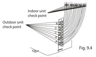
A, B,C,D are points for one-four type. A, B,C,D, E are points for one-five type.
