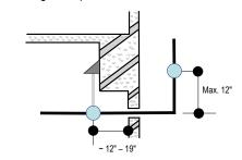
Figure 17: Pipe Support at Indoor Unit.
