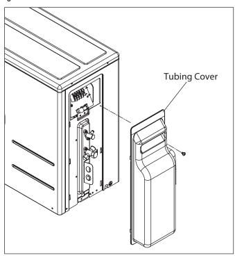
Figure 22: Heat Pump Outdoor Unit Piping Connection
