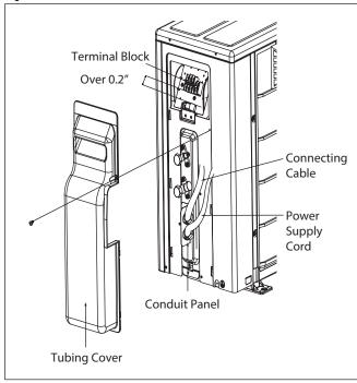
Figure 26: LSN243HLV/LSU243HLV, LSN303HLV/LSU303HLV, LSN363HLV/LSU363HLV Outdoor Unit Electrical Connection.
