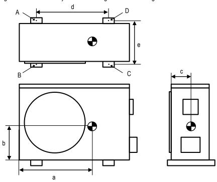
Table 5: Center of Gravity and Corner Weight Dimensions.
