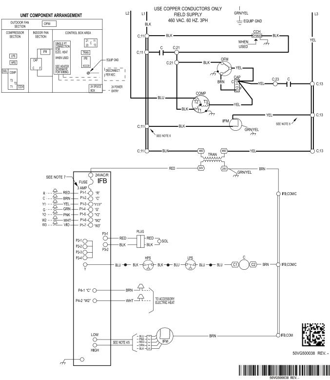
Fig. 14 Cont. - Ladder Wiring Diagram 460-3-60
