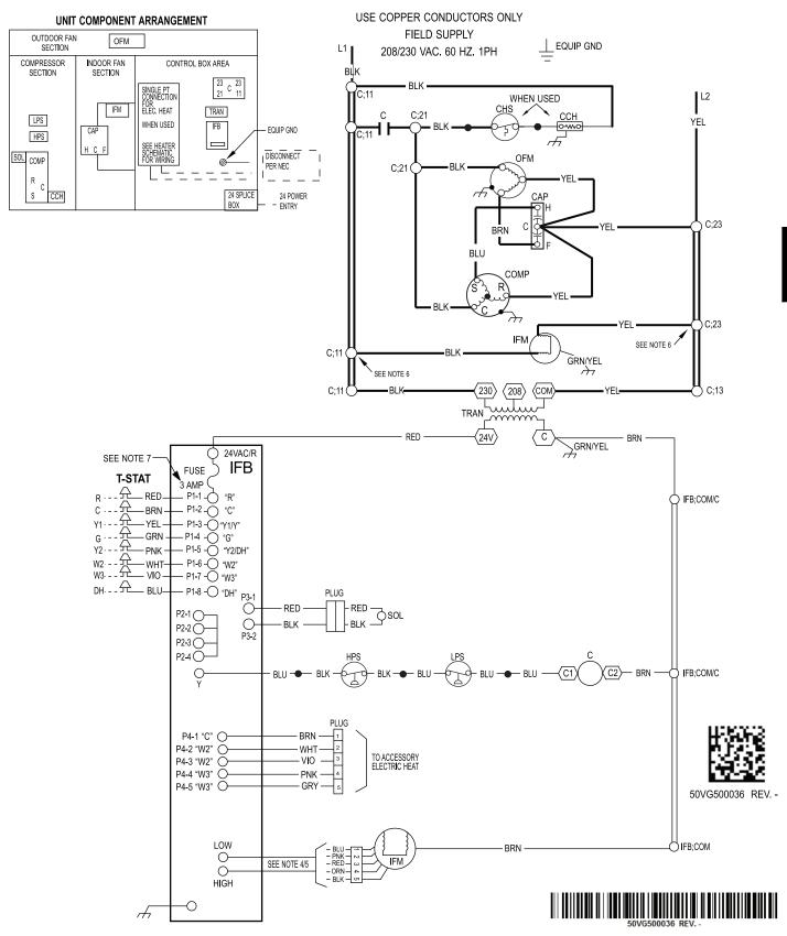
Fig. 12 Cont. - Ladder Wiring Diagram 208/230-1-60
