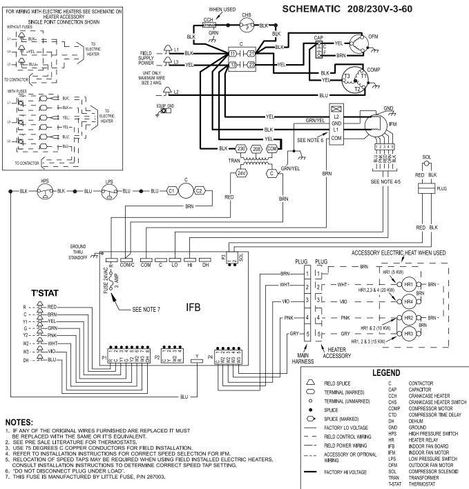
Fig. 13 - Connection Wiring Diagram 208/230-3-60
