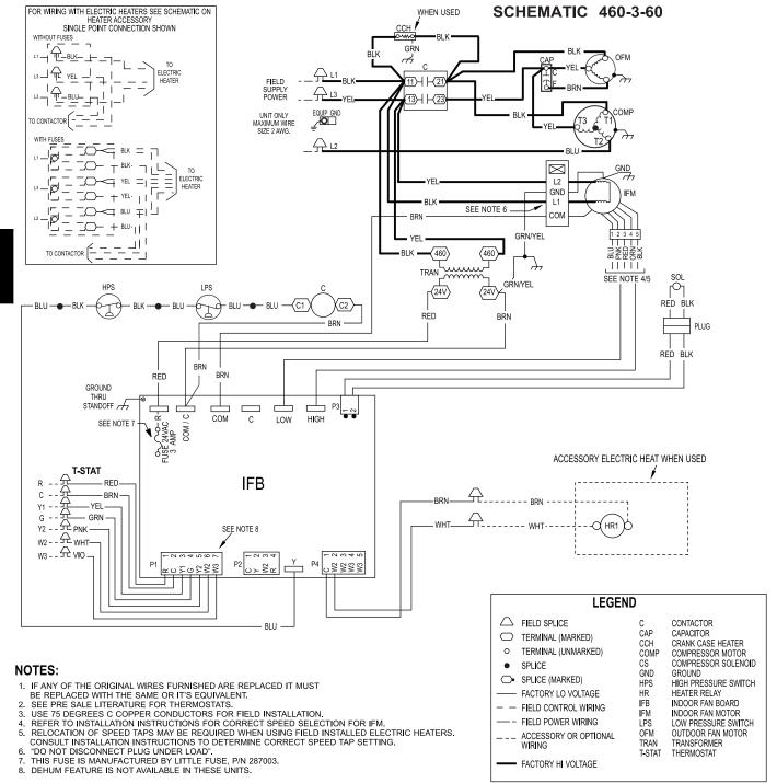
Fig. 14 - Connection Wiring Diagram 460-3-60
