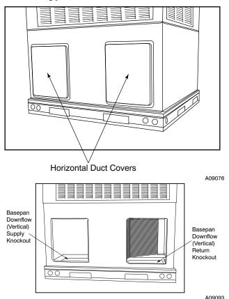
Fig. 9 - Supply and Return Duct Opening
