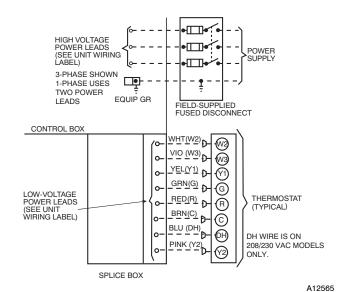
Fig. 10 - High- and Control-Voltage Connections
