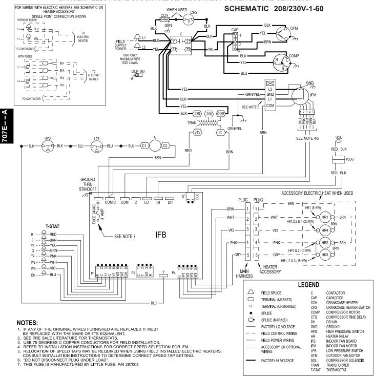
Fig. 12 - Connection Wiring Diagram 208/230-1-60
