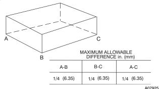
Fig. 6 - Unit Leveling Tolerances
